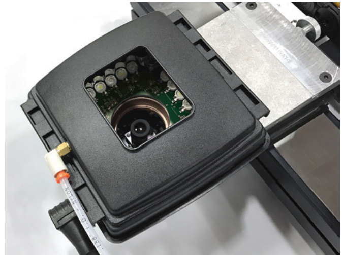
Minimize scanner cleaning with MultiCam's active OptiGuard, which uses compressed air to keep the lens clean from ink mist and dust—keeping maintenance to a minimum.
