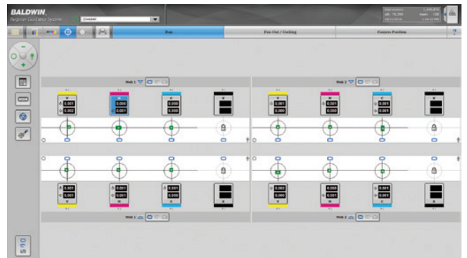
Register Guidance with MultiCam displays all print units at a glance, and the system automatically keeps your print run within established tolerances.
